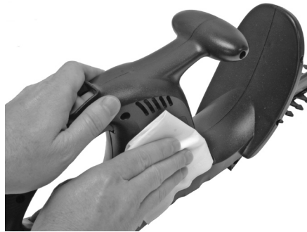
Figure 4-1: Cleaning trimmer housing
